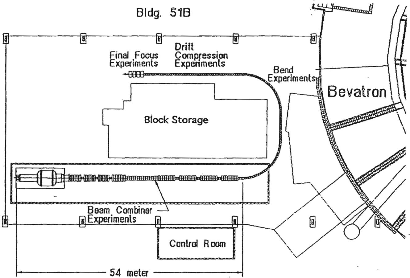
**Figure 4. Overall Induction Linac System Experiments Configuration**
