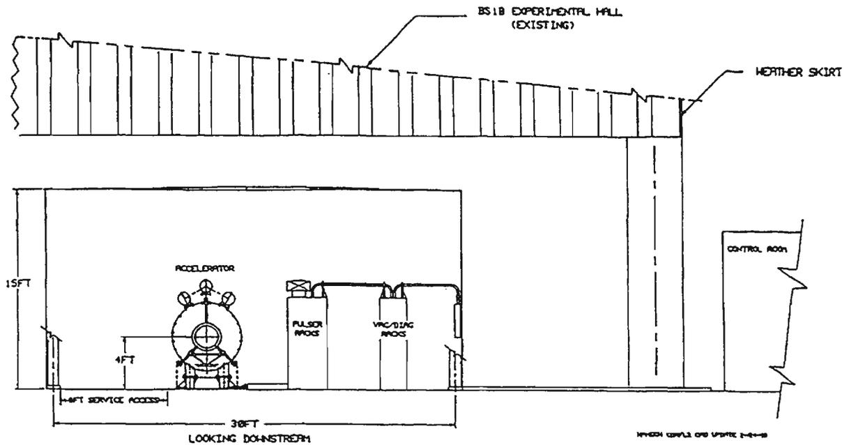
**Figure 3. Cross-section View of the Proposed Building and Accelerator Area in Relation to Existing Building 51B**
