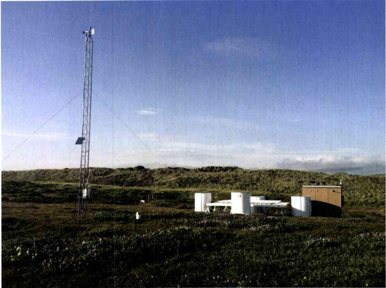
**Figure 5.** A wind-profiling equipment site currently operating at the Bodega Marine Laboratory in Bodega Bay, California. The 10 m meteorological tower is on the left, the 449 MHz wind profiler is surrounded by the RASS acoustic sources in the center, and the equipment shelter is on the right.
