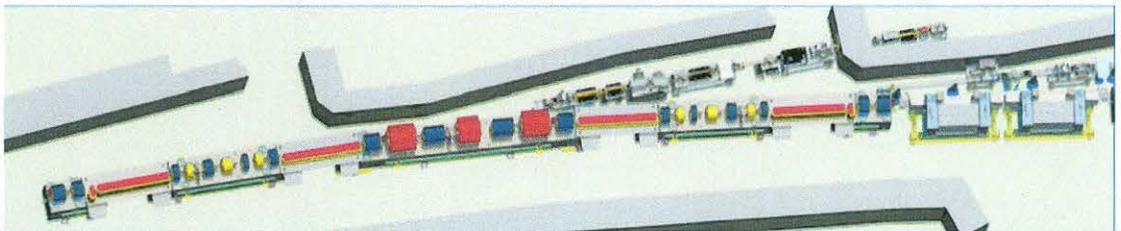
*Figure 1. A single sector of the current (top) and MBA (bottom) lattice as implemented at the APS. An insertion device would be located at the left where the graphic ends; two inline devices are shown at the right. Dipoles are red, quadrupoles blue, and sextupoles yellow. The current walls of the storage ring enclosure are shown in both depictions*
