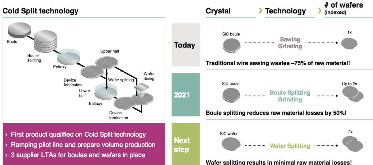
**Figure 12:** Infineon Cold Split technology
