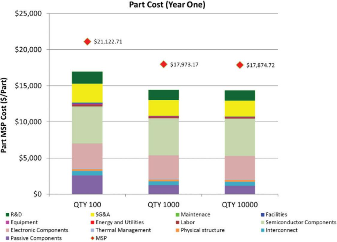
**Figure 9:** Modeled factory gate pricing of Alpha SiC inverter
