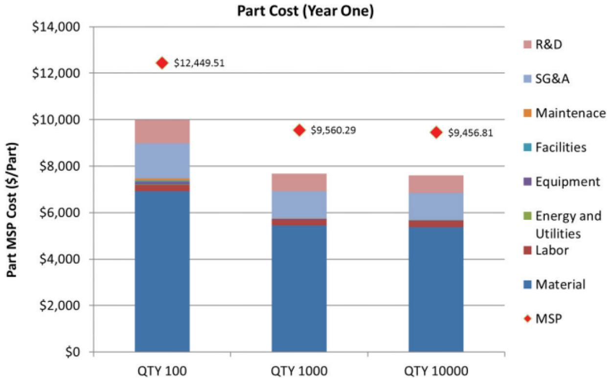
**Figure 10:** Modeled factory gate pricing of Gamma SiC inverter using current die pricing.
