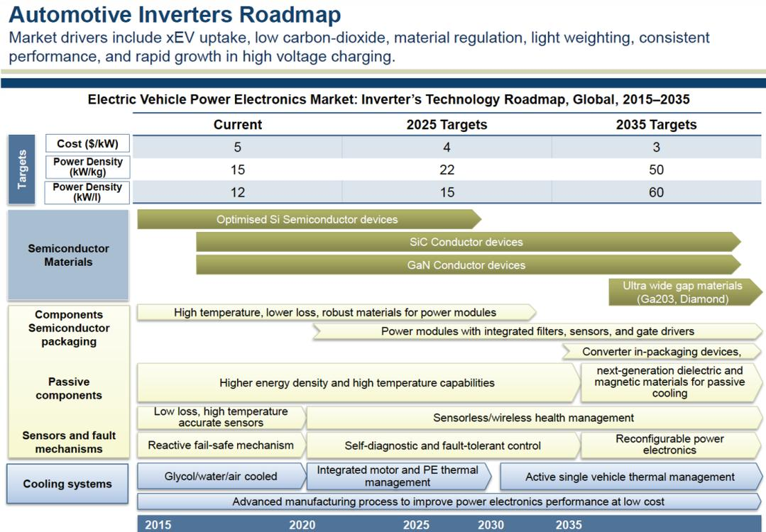
**Figure 4:** Roadmap for Automotive Power SiC / GAN Devices
