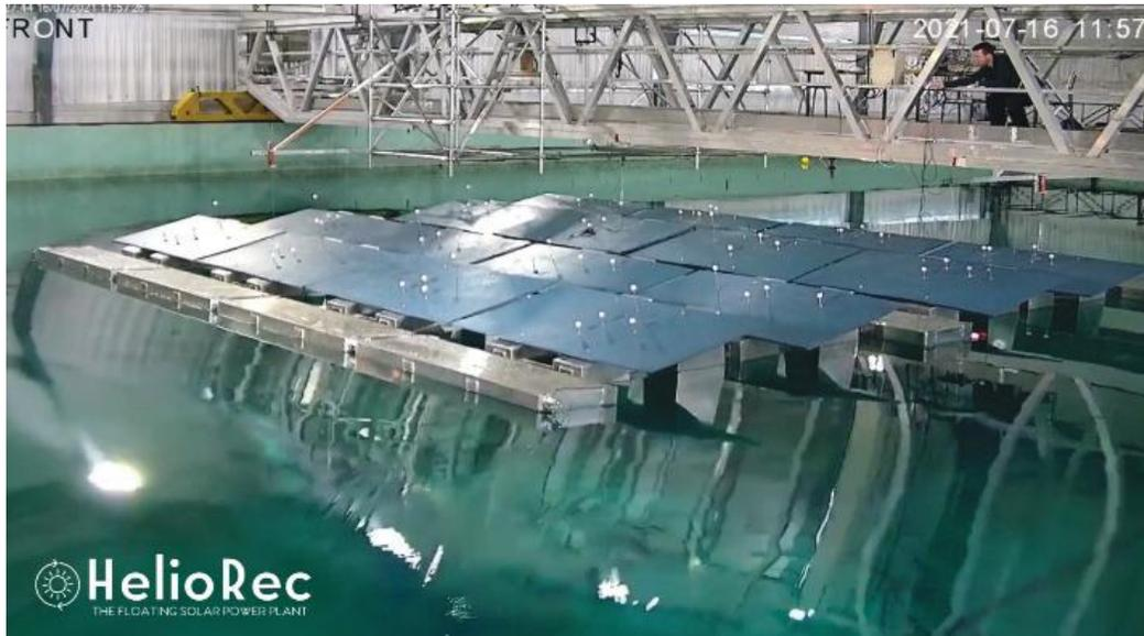
**Figure 14:** Heliorec Wave Tank Testing
