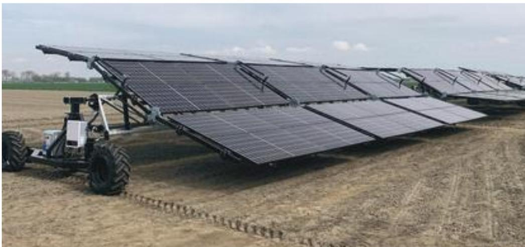
**Figure 9:** The mobile agrivoltaics array
