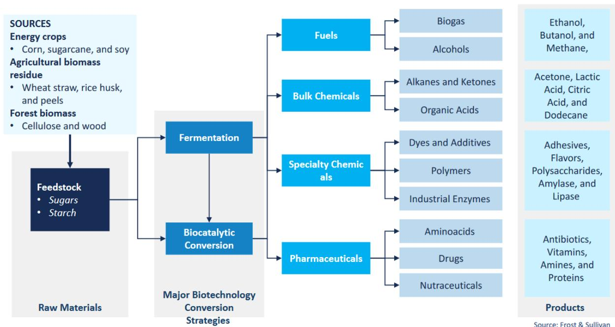
**Figure 2: Process of Chemical Transformations of Substrates into Products and Sources of Biomass**
