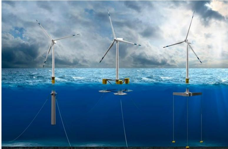
**Figure 4:** Illustration of floating foundation types (NREL 2022)
