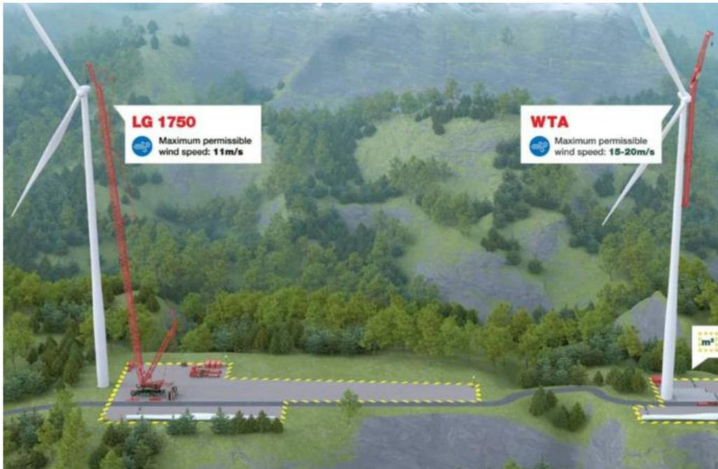
**Figure 15:** Comparison of Mammoet WTA and Liebherr LG 1750 Lattice Boom Mobile Crane
