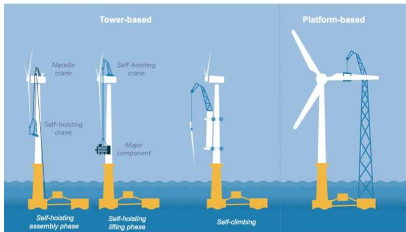
**Figure 7:** Tower-based and Platform-based Add-on cranes
