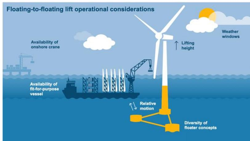
**Figure 6:** Lifting needs when transferring from one floating entity to another
