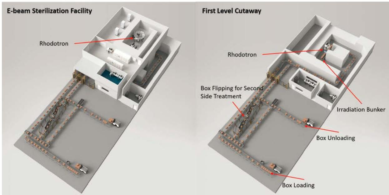
**Figure 4:** Prototypical E-beam Sterilization Facility<sup>8</sup>
