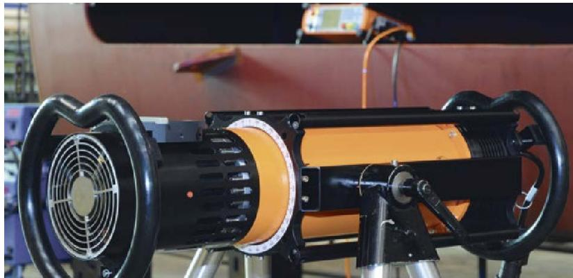
**Figure 21:** Seifert ERESO MF4 Portable Industrial X-ray Generator
