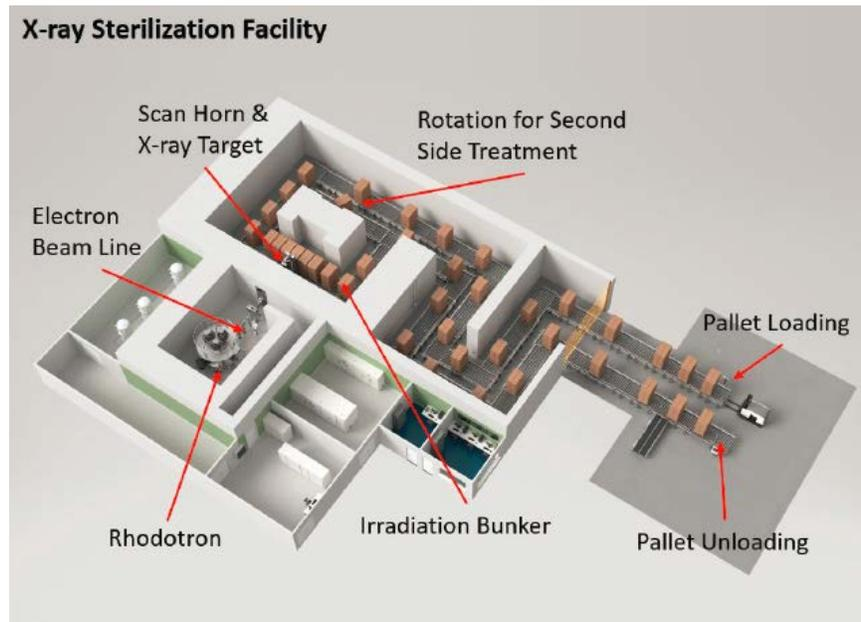
**Figure 3:** X-ray Sterilization Facility<sup>6</sup>
