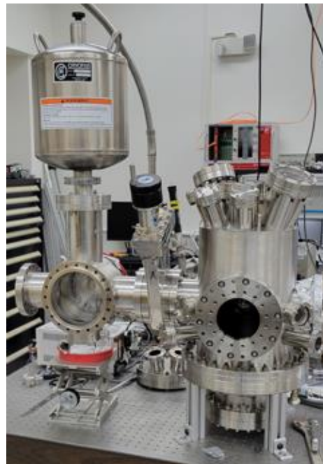
Figure 3 – A DC magnetron sputtering system for depositing thin film coatings. This system will be used to prepare magnetostrictive thin films on silicon substrates needed to test the Mag-MEMS concept.
