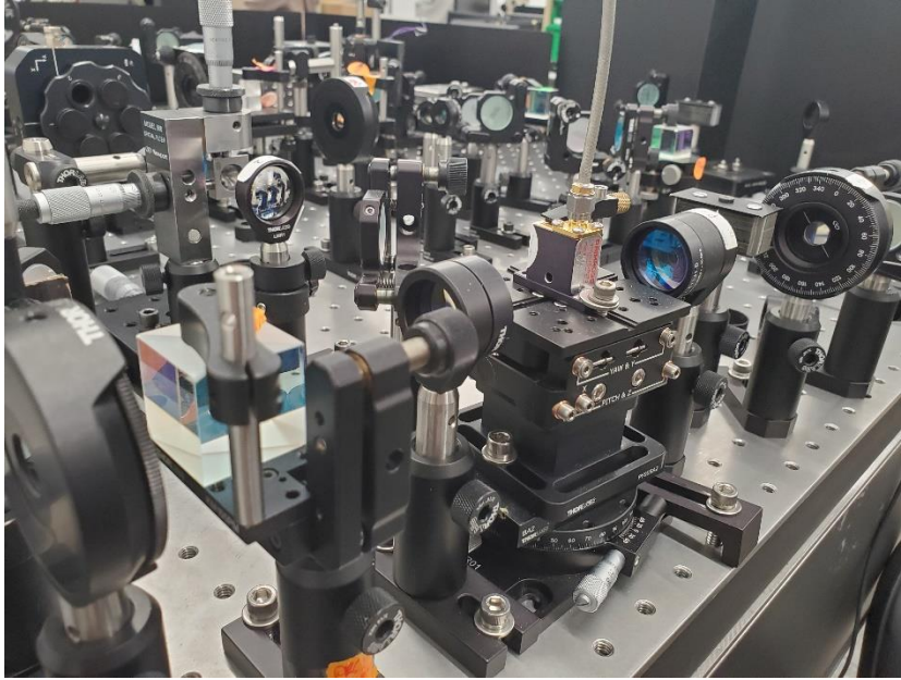
Figure 4: Optical components of the squeezed light source placed on a portable breadboard. In the foreground an acousto-optic modulator is shown in a double-pass configuration. The double-pass diffraction efficiency was tuned to 3% for about half of the nominal input RF drive power capacity, providing ample headroom of hundreds of microwatts available in probe power. The device provide a probe field by frequency-downshifting a field by 1.5GHz into the first order output, twice, for an effective downshift of 3GHz, obtaining the needed energy separation shown in Fig. 1c. The resultant fields are then sent to the rest of the optical train shown in the background, leading the Rb vapor cell.
